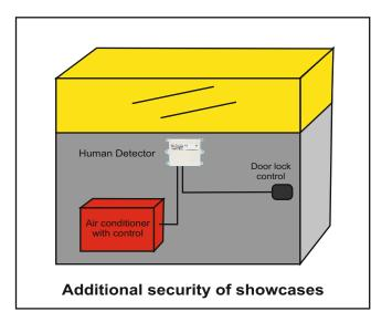
Please be aware that there is a risk of accidental activation in highly vibrating floors. The sensitivity should be reduced in this case. If necessary, the external alarm input is then connected to potential additional sensors, e. g. a switch for closing control, the alarm output of the air conditioning system or the connection of the "glass spider".
