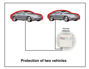
**heddier electronic GmbH** Raiffeisenstraße 24 48734 Reken, Germany A second vehicle can also be connected to the reference input instead of the metal plate. This secures both automobiles. It is recommended to additionally switch on the seismic sensors for objects with larger, non-conductive surfaces. The exact procedure is described in the manual.
