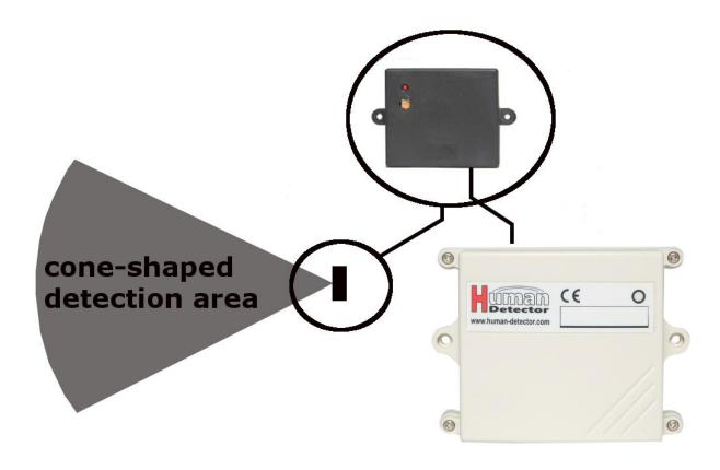
The external radar sensor (article: RS-1Z) from heddier electronic GmbH can be connected via this interface. Its compact design and the ability to easily penetrate non-conductive material allows for the simple, fast and concealed installation. Movements of persons are detected in the cone-shaped detection area up to a distance of 2.5 meters. The range can be directly controlled at the sensor.
