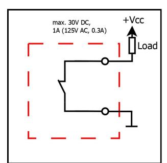
**Note:** The connection of external devices to the NC relay output should be carried out by qualified personnel. A faulty connection can lead to the destruction of the device.
