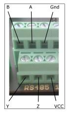
The full duplex RS485 interface can be used to control external devices, especially surveillance cameras. The interface parameters as well as separate commands (up to 12 byte) can be set in the **Human Detector** software.
