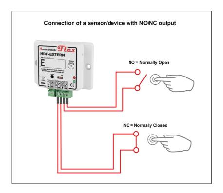
Sensors with open-collector outputs can also be connected directly. For this purpose, an additional 470 kOhm resistor needs to be connected between the sensor input and the operating voltage +U B. It may be necessary to adjust the resistance value, depending on the design of the external sensor.
