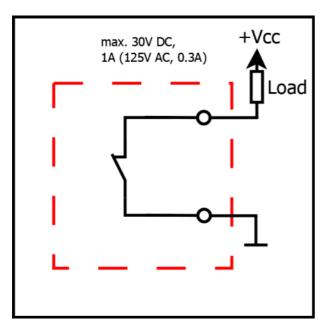
**Note:** The connection of external devices to the NC relay output should be carried out by qualified personnel. A faulty connection can lead to the destruction of the device.
