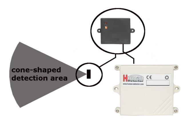
The external radar sensor (article: RS-1Z) from heddier electronic GmbH can be connected via this interface. Its compact design and the ability to easily penetrate non-conductive material allows for the simple, fast and concealed installation. Movements of persons are detected in the cone-shaped detection area up to a distance of 2.5 meters. The range can be directly controlled at the sensor.
