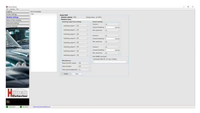
You can set the performance of the module in the event of an alarm in system menu "Module Settings". You can also give the **Human Detector** Module there a clear name (see page 24 "System Menu / Module Settings").
