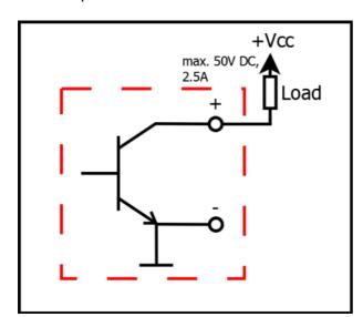
**Note:** The connection of external devices to the switching outputs OC should be carried out by qualified personnel. These are semiconductor switch outputs. A faulty connection can lead to the destruction of the device.
